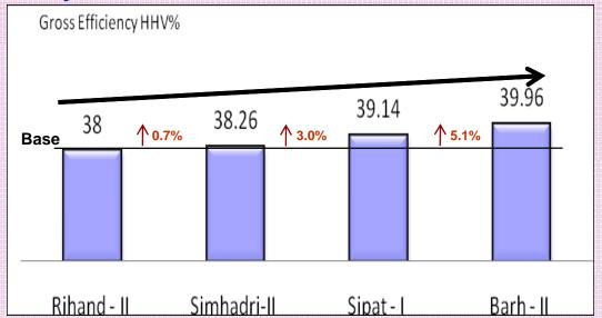
Study for adopting ultra-supercritical technology with efficiency levels of 41.1% in progress.
