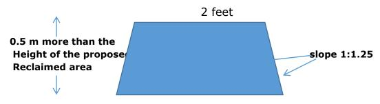
**Cross- section of water body protection embankment**
