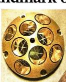
NASA's Laser Retroreflector Array on Vikram lander. NASA's Goddard Space Flight Centre
