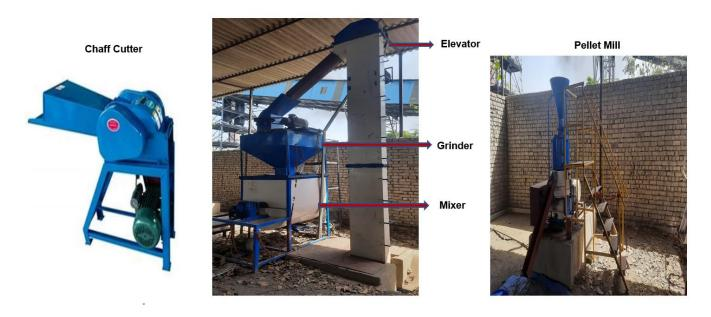
Biomass pellet machine having a capacity of 250 kg/hour has been installed for Agricultural/Forest Waste management to address the issue of stubble burning. The agriculture/forest waste is collected and mixed with molasses to upcycle into pellets. These upcycled pellets are then blended with coal in the combustion process which reduces greenhouse gas emissions.
