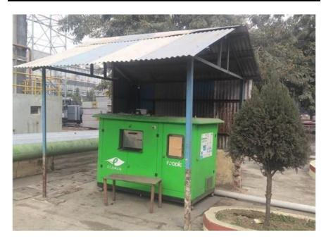
125 kg/day capacity Organic Waste composting 'FOODIE' machine has been installed for sustainable management of biodegradable waste generated from plant canteen.
